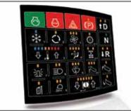
Convenient sealed switch module provides fingertip control of numerous productivity enhancing functions including: **Keyless Start, I-Tip, Dump Body Upper Limit, Soft Stop/Hard Stop Selection, Retarder Aggressiveness and Speed Control.**
