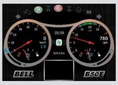
A user friendly 10" colour monitor offers vital operating information, safety warnings, detailed diagnostic readings and dump body function settings.
