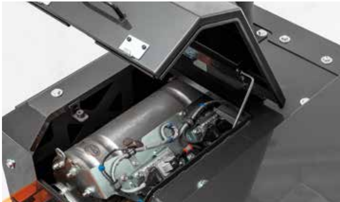
Service intervals for the CSF filter have increased from 4,000 to 6,500 hours.
