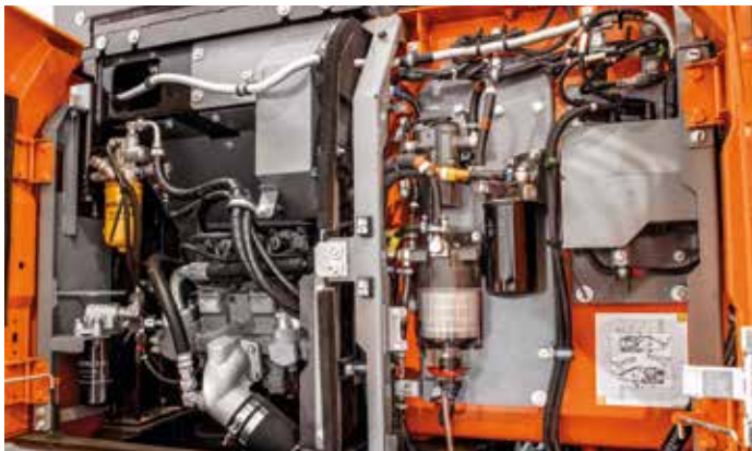
Filters have been repositioned for easy access.
